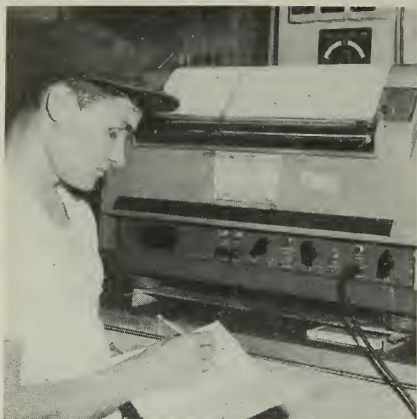
ON THE BEAM —Positive Depth Recorder sends electronic radio beam to ocean's floor and records depth of sea.
